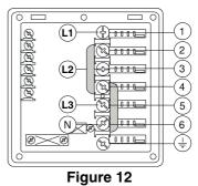
Open the power supply terminal board and insert the jumpers provided as follows: one jumper between terminals 2 and 4 and another between terminals 4 and 6. Using a suitable power supply cable (see technical data table), connect the three phases to terminals 1, 3 and 5, the neutral to terminal 4 and the earth wire to the terminal  $-\frac{1}{2}$ .
