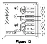
Open the power supply terminal board and insert the jumpers provided as follows: one jumper between terminals 1 and 2, one between terminals 3 and 4 and another between terminals 5 and 6. Using a suitable power supply cable (see technical data table), connect the three phases to terminals 1, 3 and 5 and the earth wire to the terminal  $\frac{1}{2}$ .
